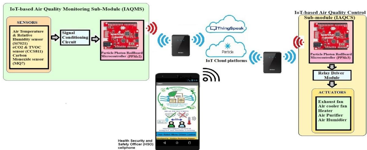
Fig. 3. IoT-based Air Quality Monitoring and Control System Block diagram
