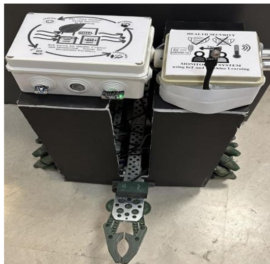
Fig. 2. Mecanum-wheeled Autonomous Robot for Hotel and Other Hospitality Facilities (MAROH)
