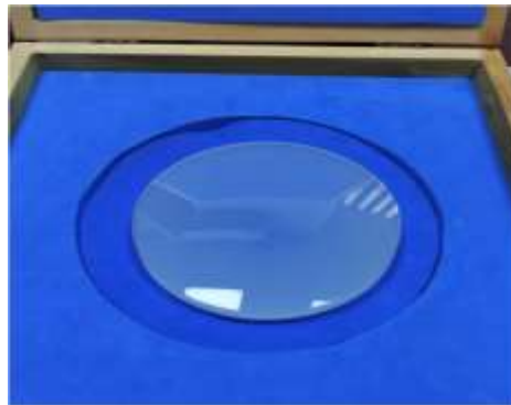
Figure 8: Photo of fabricated precise BK7 aspheric lens
