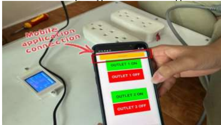
Figure 3.17 Prototype and Android Application's Bluetooth Connectivity
