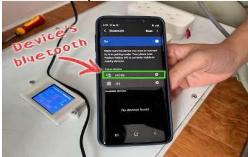
Figure 3.16 Bluetooth Connectivity between Prototype and Mobile Phone
