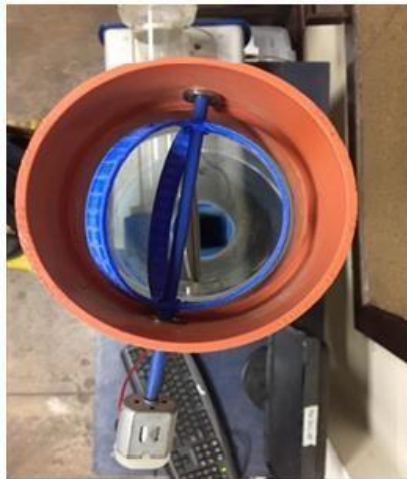
Fig. 6. Three-bladed Globe-type Darrieus wind turbine set-up
